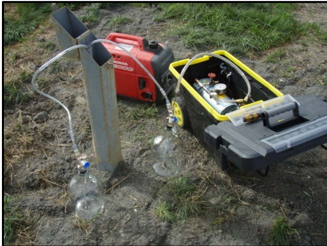
Figure 2: A vacuum pump applies suction to soil lysimeter probes buried in the soil, drawing soil water for analysis.
