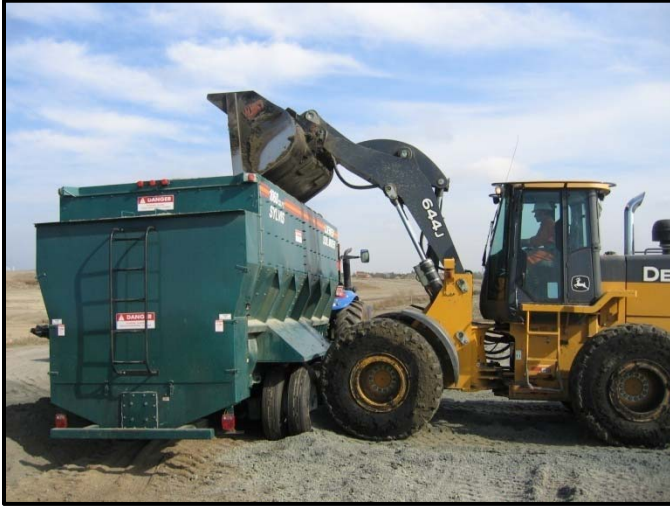
Figure 1: Wheel loader adds feedstock ingredients to the SYLVIS soil mixer based upon a volumetric ratio.
